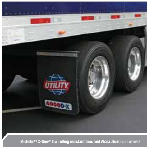
Michelin® X-One® low rolling resistant tires and Alcoa aluminum wheels
