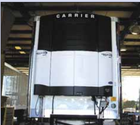
Factory installed refrigeration unit
