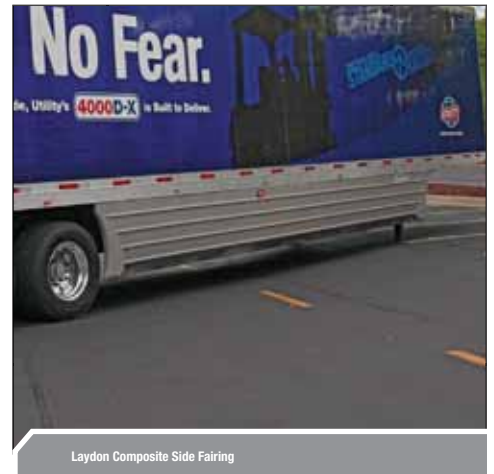
Laydon Composite Side Fairing
