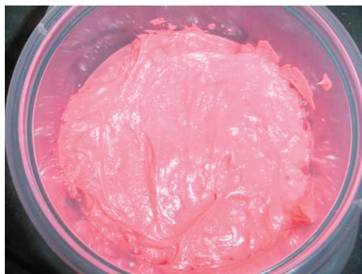
Figure 2: Red/pink semi-fluid grease contaminated with a small amount of water turns milky pink.
