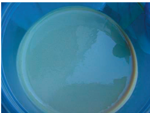
Figure 1: 50 weight synthetic oil contaminated with a small amount of water turns milky white.
