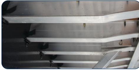
39,000 lb coil haul package with a 5 foot span of 4" tapered to 3" aluminum crossmembers on 8" centerlines to provide optimized strength at the coil.
