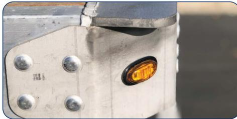
Stainless steel corners and top plates protect against impact damage and provide additional strength and durability, reducing cost of ownership.
