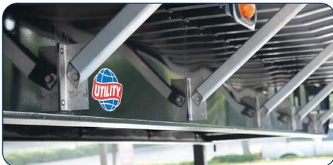
Five tube-shaped outriggers located on each side of the flatbed are connected to the crossmembers, providing stability and helping distribute the load to the main beams.
