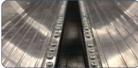
The 80K steel hat-shaped top flange provides added lateral stability, adding to a longer trailer life.
