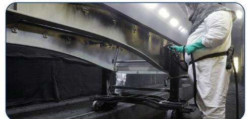
The main beams are shot blasted to bare metal prior to painting and then coated with a two-part primer and two-part urethane top coat on the exterior surfaces. A rust preventative coating is applied to the interior surfaces of the beams for lower maintenance costs.
