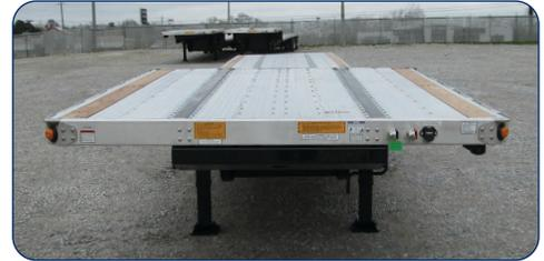
Designed to lower tare weight, this high strength aluminum front rail provides added protection, improves durability, and reduces maintenance expenses.
