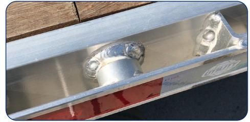
The aluminum side rail has an integral winch track and heavy-duty pipe spools. The pipe spools are engineered to a 6,500 lb working load limit rating.
