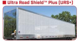
ASTM proven, this two coat acrylic system with urethane primer enhances corrosion protection, minimizes the effects of weathering and keeps the trailer looking better, longer.
