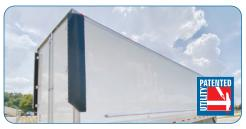
Comprised of two black side foils and one single black top foil assembly, the side foils are connected to the swing doors and will deploy and un-deploy when the doors are opened and closed.
